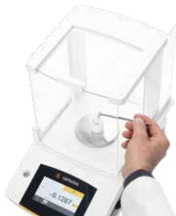
Fig. 4: Applying accelerator to a weighed sample
