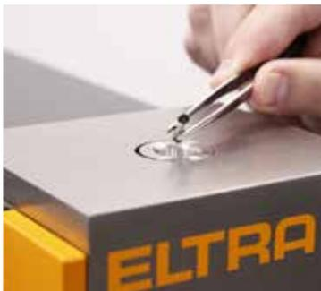
Fig. 9: Application of open capsule with powder
