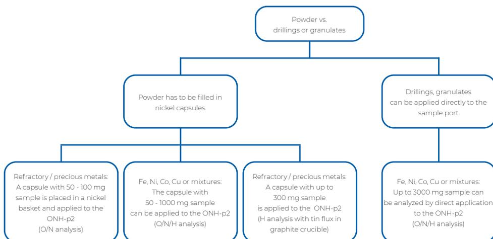
The separation between powders and drillings is not defined clearly.
